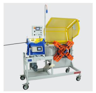
This small but effective electrical ring coiler are primarily used by electrical wholesalers and industry. It is intended for the frequent and professional winding of smaller cables, wires or lines from delivery drums onto rings. Using a spool as an accessory, lengths of cable can also be rewound from larger drums to smaller ones.
